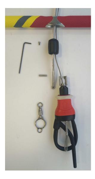
9) Put your new pin (5x22) back into the QR, but through the Depower Line hole.
