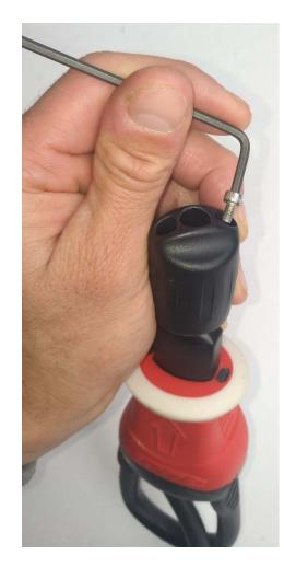
5) Remove the Line Twister, and the pin (5x22mm) that is into it (no need of any particular tool).
