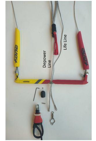
7) Pass your new Depower Line and Life Line through the 2 holes of the Line Twister, as shown below : Depower Line in the center hole.
