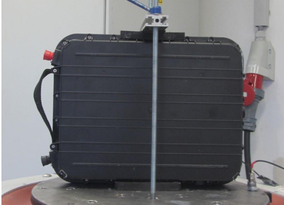
Figure 20: Specimens fitted towards Y Direction (test procedure conducted in several parts)
