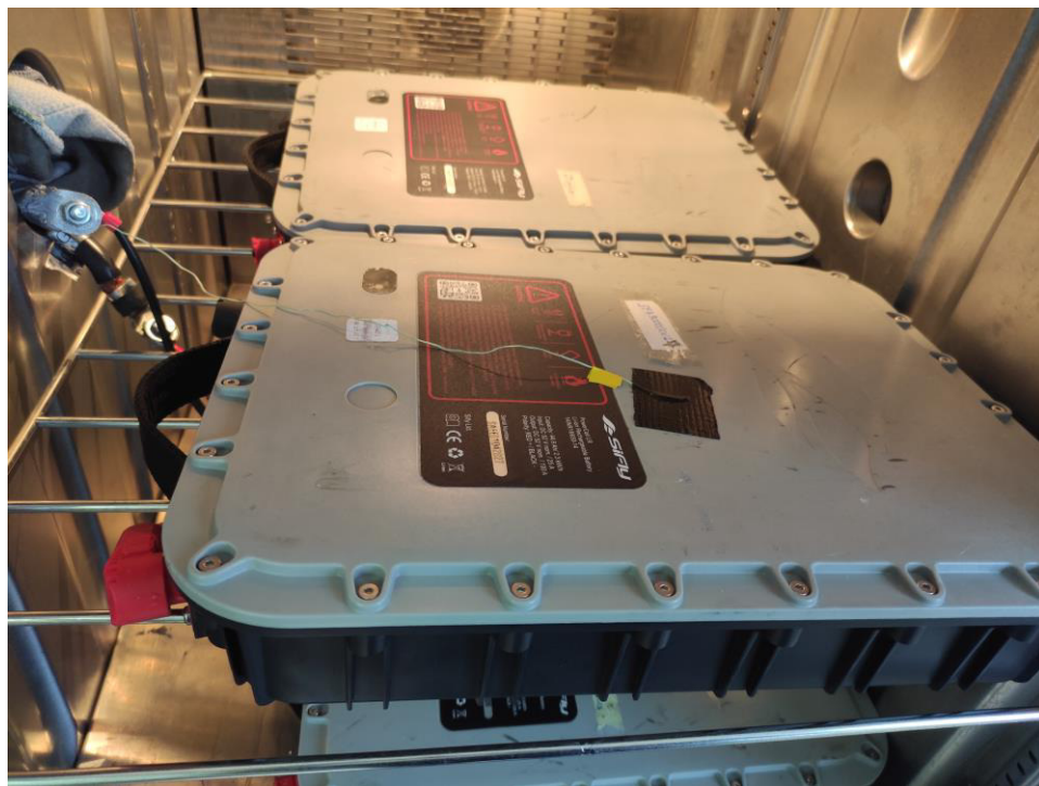
Figure 29: Specimens inside temperature test chamber
