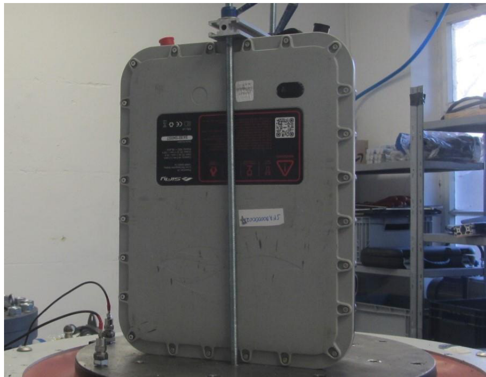
Figure 19: Specimens fitted towards X Direction (test procedure conducted in several parts)
